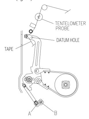
Fig.46 BACK TENSION MEASUREMENT
